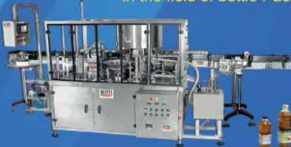
Multi Utility Labeling Machine for Square, Hexagonal, Octagonal & Round Bottles(50BPM to 400 BPM)
