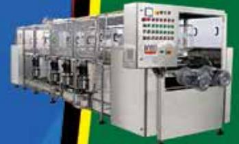
Automatic Jar Washing, Machine 7 Stages with outside Jar brushing and Automatic unloading
